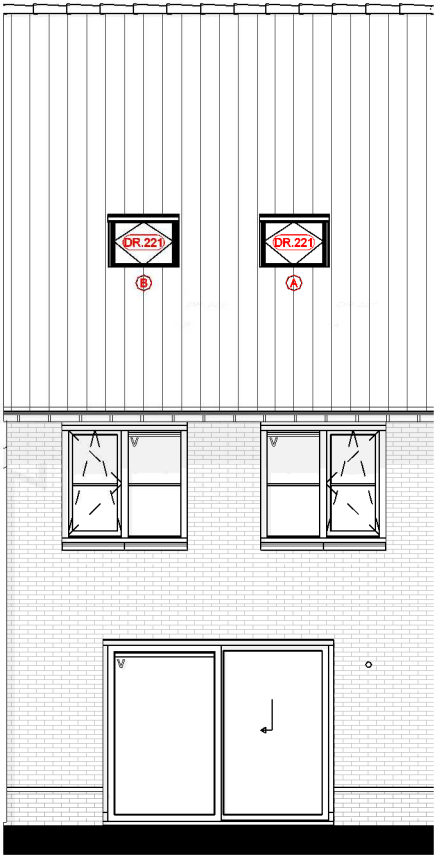
Achtergevel DR.221 = Extra houten tuimeldakraam (ca.980 x 940mm)
