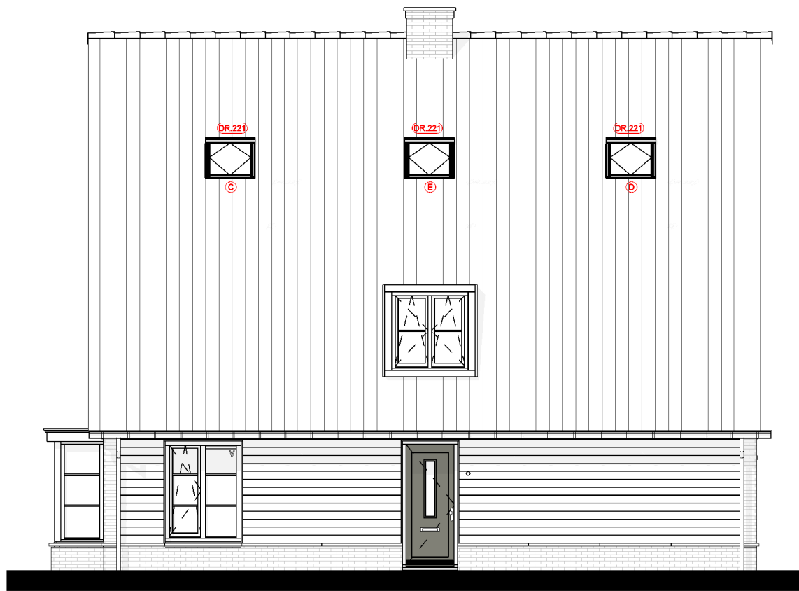
Rechtergevel DR.221 = Extra houten tuimeldakraam (ca.980 x 940mm)
