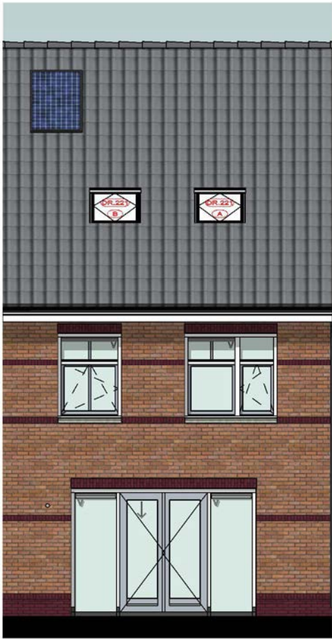
Achtergevel DR.221 = Extra houten tuimeldakraam (circa 980 x 940 mm)
