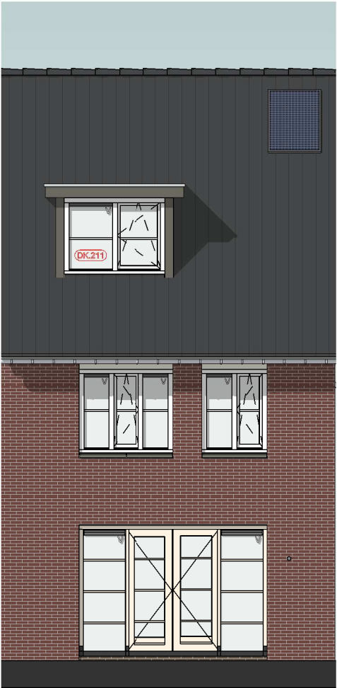
achtergevel DK.211 = Dakkapel ca.1800mm
