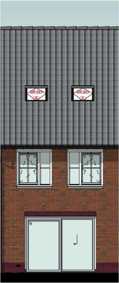
Achtergevel DR.221 = Extra houten tuimeldakraam (circa 980 x 940 mm)
