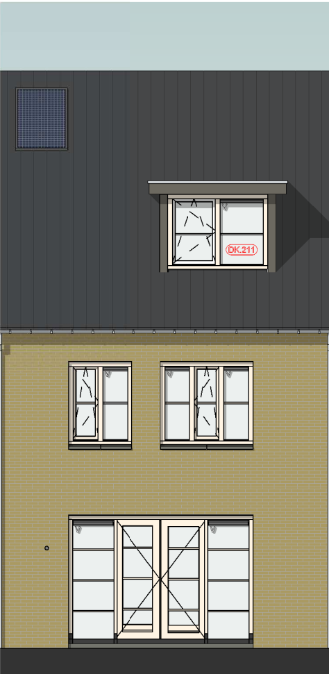
achtergevel DK.211 = Dakkapel ca.1800mm
